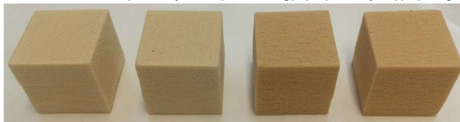
Polyurethane foam samples containing polyols produced from pyrolytic sugars
