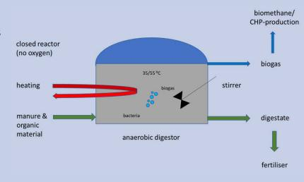
One way to enhance the production of biogas is to mix other organic substances with the feedstock. Sometimes, these additives can make up half of the input volume. The resulting material after digestion, called digestate, can be applied as a biofertilizer.
